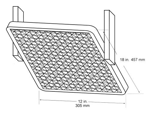
Figure 3b – Air Propane Radiant Panel
