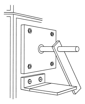
Figure 8 - Propane Burner Stop
