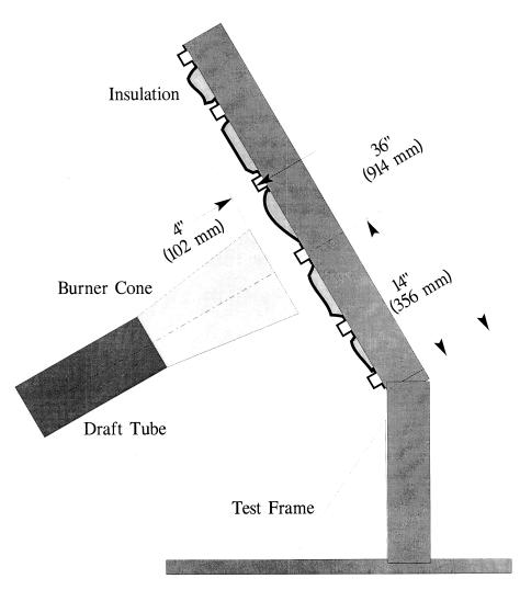
Figure 2 – Burnthrough Test Apparatus
