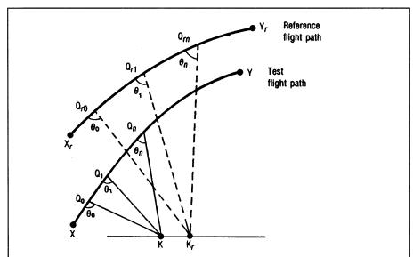
Figure A36-10. Correspondence between measured and reference flight paths for the application of the integrated method of adjustment
