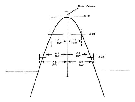
NOTES: 1. The beam envelope is smoothed by a 26 kHz video filter before measurement.
