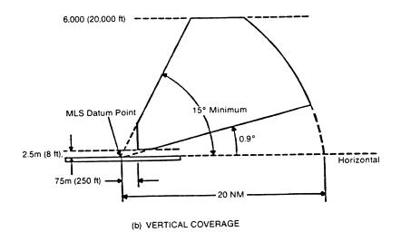
Figure 13. Approach Elevation Coverage
