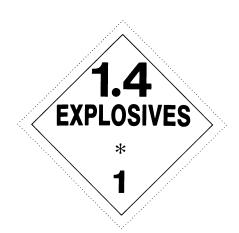
(b) In addition to complying with §172.519 of this subpart, the background color on the EXPLOSIVES 1.4 placard must be orange. The "\*" shall be replaced, when required, with the appropriate compatibility group letter. The division numeral, 1.4, must measure at least 64 mm (2.5 inches) in height. The text, numerals and inner border must be black.
