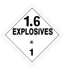
(b) In addition to complying with §172.519 of this subpart, the background color on the EXPLOSIVES 1.6 placard must be orange. The "\*" shall be replaced, when required, with the appropriate compatibility group letter. The division numeral, 1.6, must measure at least 64 mm (2.5 inches) in height. The text, numerals and inner border must be black.
