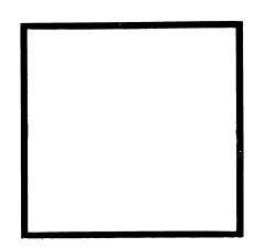
(b) In addition to meeting the requirements of §172.519 for minimum durability and strength, the square background must consist of a white square measuring  $14\frac{1}{4}$  inches (362.0 mm.) on each side surrounded by a black border extending to  $15\frac{1}{4}$  inches (387.0 mm.) on each side.
