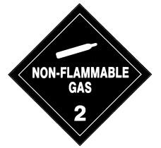
(b) In addition to complying with §172.519, the background color on the NON-FLAMMABLE GAS placard must be green. The letters in both words must be at least 38 mm (1.5 inches)
